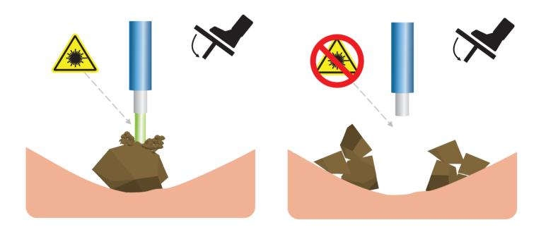
The principle of the Tissue Sensor is that the laser detects which tissue (hard or soft) is in front of the surgical fiber tip.
