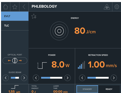
In "Phlebology" mode, the energy is automatically calculated based on the selected power and retraction rate parameters
