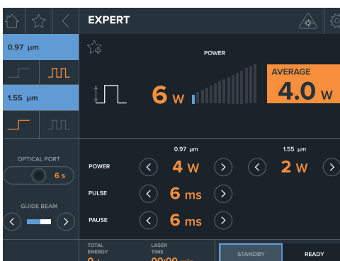
In "Expert" mode FiberLase S allows for controlling two independent radiations (0.97 and 1.55 \mu\text{m} ) through one fiber instrument
